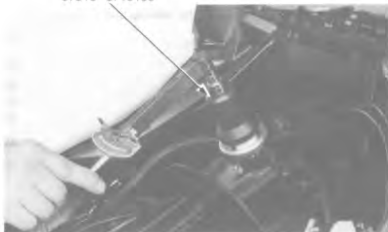
STEERING STEM SOCKET 07916–3710100
