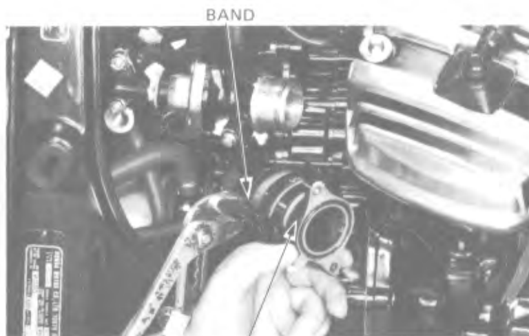
INLET PIPE JOINT
