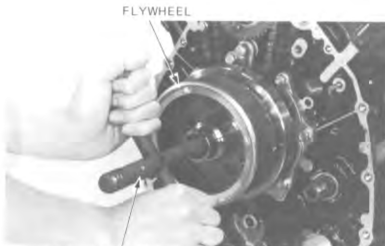
FLYWHEEL PULLER, 20 mm 07933-3950000 OR 07733-0020001
