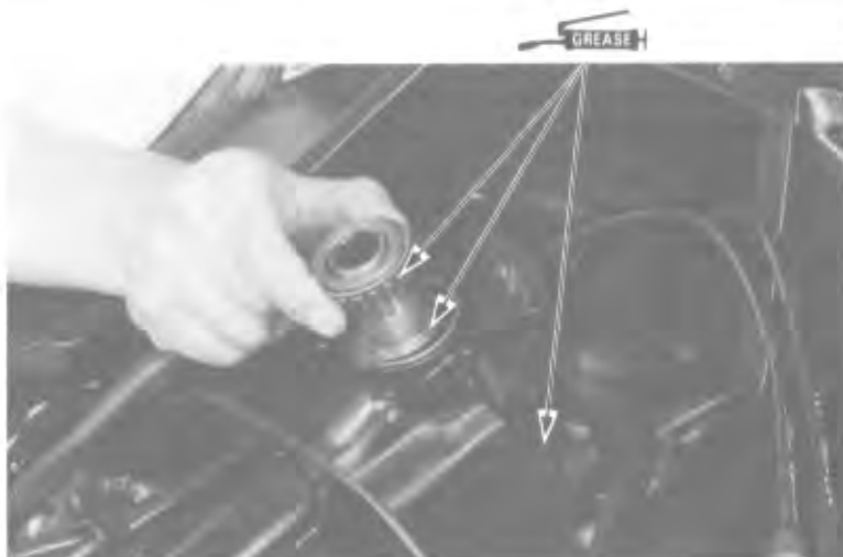
STEERING STEM SOCKET 07916–3710100
